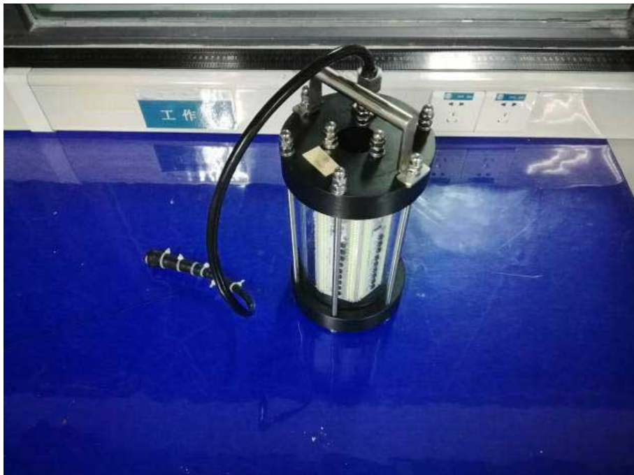
Photo 4: the sample after the IPX8 test
