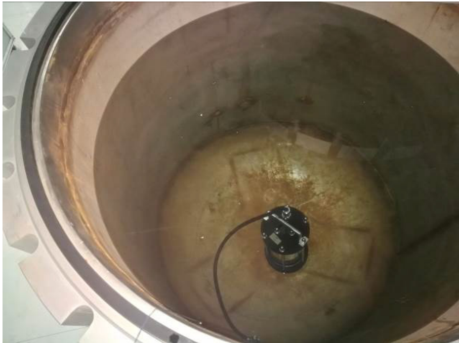
Photo 1: the sample inside the IPX8 Test Pressure Vessel
