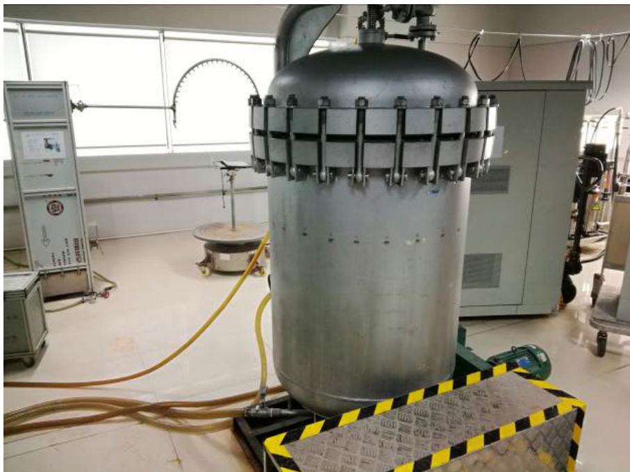
Photo 2: the IPX8 test in progress
