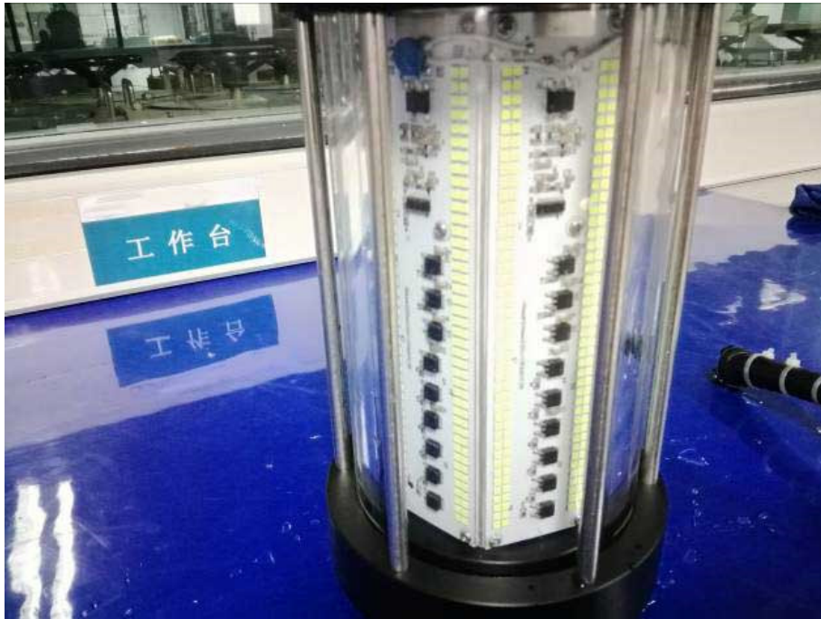
Photo 5: the sample after the IPX8 test
