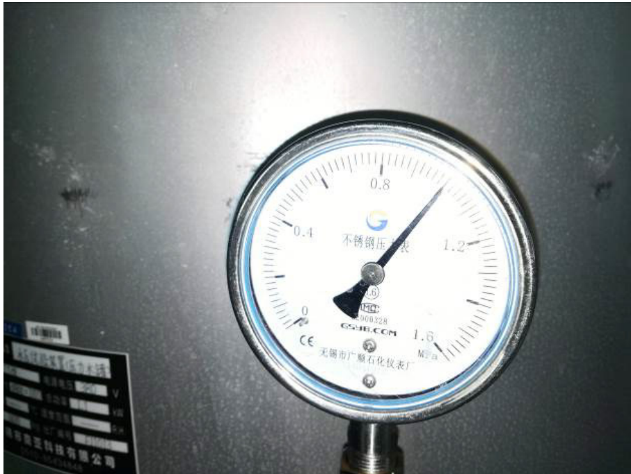
Photo 3: the IPX8 pressure monitoring
